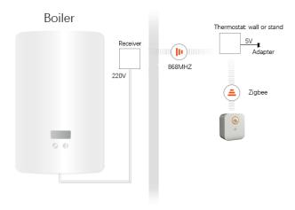
The thermostat control wirelessly the boiler through the receiver. The receiver directly connect to the boiler by wires. The thermostat is powered by the adapter.
