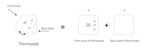
Then use the front cover of thermostat mounted on the back plate of the receiver. As shown in the picture below:
