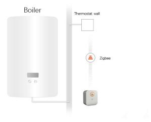
The thermostat control directly the boiler and get power supply through the reserved wirings.
