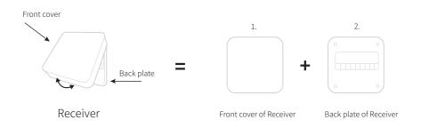
Separate the front cover and back plate of the thermostat.
