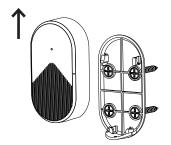
3. Mount the main unit onto the wall mount bracket. After installation, secure it with screws at the bottom to prevent unauthorized removal.
