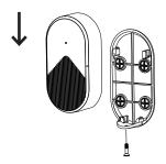
4. Remove the cap from the magnetic strip and secure it in place using screws.Replace the cap after completing the installation.
