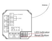
\* The product is only for In-door use. The depth of the bottom box should be over than 60 mm. Professionals are required to install or dissemble the product.
